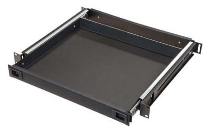
The **9041** sliding shelf features high quality ball bearing slides, two latches to prevent shelf from extending at unwanted times. 50 pound weight capacity and fits in one rack space. Great for turntables, drum machines, mounting of items not equipped with rack ears. Note: Rear rack rails required
