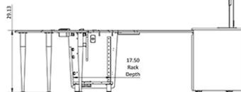
The **VC-TABLE T4 Package** consists of 1x **VC-TABLE** + 2x **CR3000EX** credenza + 2x **PM2-S** or 2x **PM2-S-XL** monitor mount. VC-TABLE T4 provides up to 82 rack units. Designed primarily for the telepresence market, this table features cable management and grommets/cubby's for easy plug in of laptops or USB keys and displaying on screen. The VC-TABLE built-in equipment rack can house a codec or PC with ten rack units easily accessible from front and rear.
