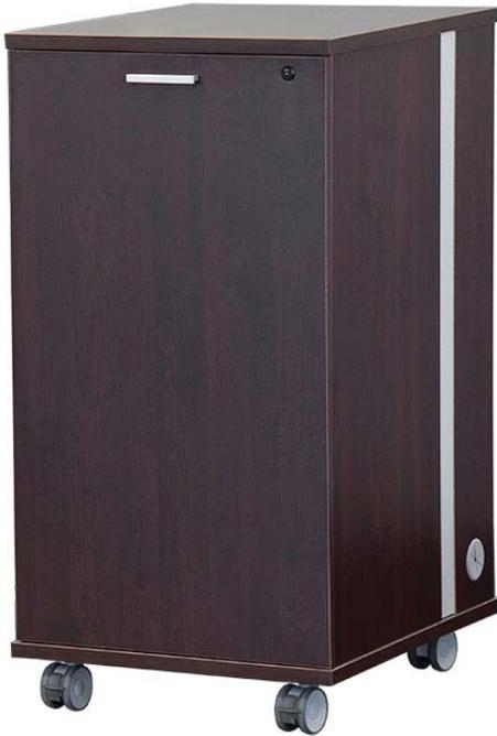
**RKYZ21** is a 21U mobile rack made with furniture grade laminates and stylish aluminum grid alongside panels. It features front 21U rack rails for equipment storage accessible from the audience side and also the presenter's. Front and rear locking doors. It offers cable access on both sides and bottom through grommets and it stands on modern casters (front two lock). This unit is an excellent addition if you want to storage equipment onto the PDYZ38 podium.
