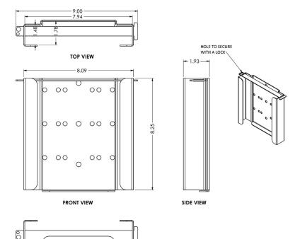
The **BKT-MCM** Mac Mini bracket allows you to easily install your Mac Mini Apple small desktop computer or other similar devices. Its design securely attaches onto our products or it can be wall mounted. Constructed from durable steel and powder coated black. Padlock not included.
